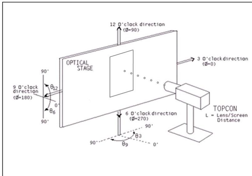
Figure 2. White Luminance and Uniformity Measurement Locations (9P point)
