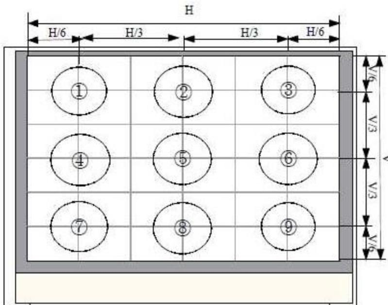
**Figure 3. Uniformity Measurement Locations (5/13 points)**
