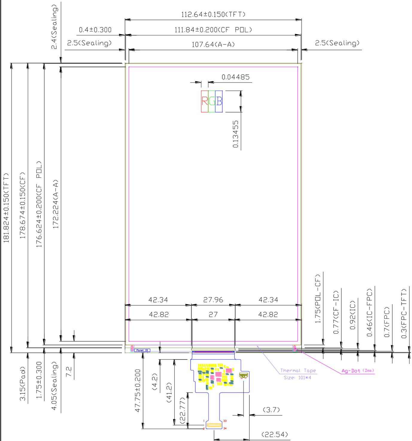
**Figure 6. TFT-LCD Module Outline Dimensions (Rear view)**
