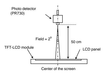
Optical characteristics measurement setup
