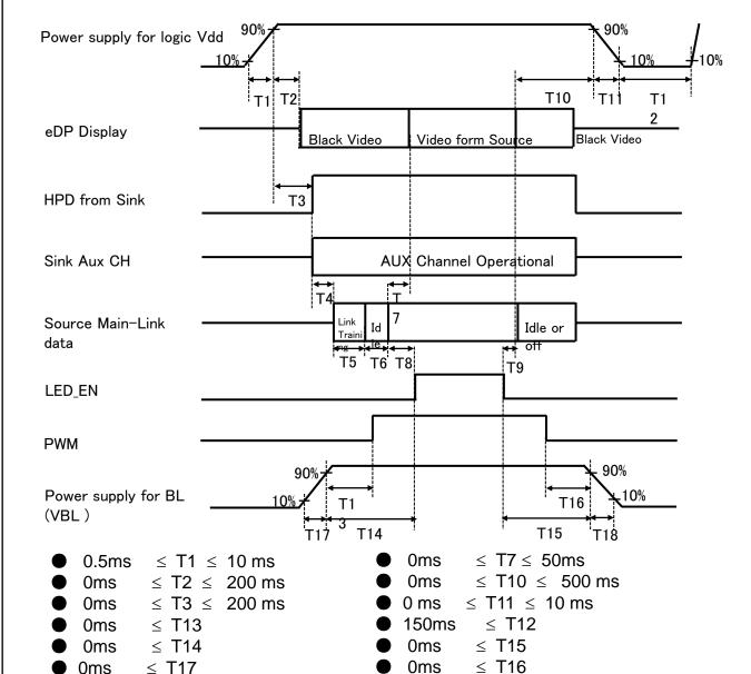
1. When the power supply VDD is 0V, keep the level of input signals on the low or keep high impedance.
